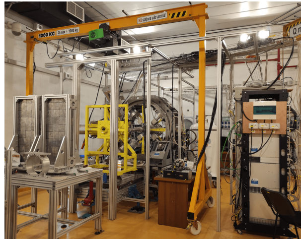
Figure 4.3.4: The present view of the ELIADÉ \gamma -ray spectrometer installed at the E8 experimental area.
