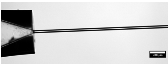
Figure 1.12.2: Image of the conical nozzle and the microjet recorded with the Leica microscope.
