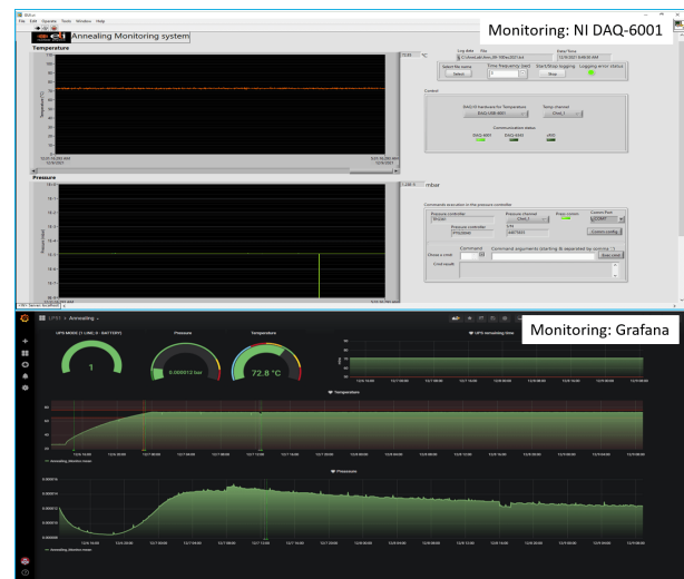
Figure 4.9.3: Screen captures of online monitoring displays for NI DAQ-6001 (upper panel) and Grafana (lower panel).
