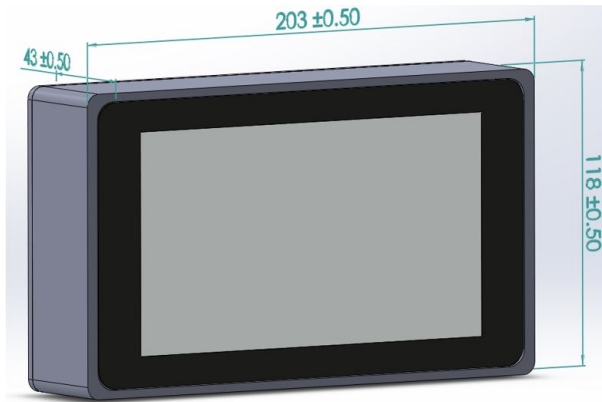
Figure 1.7.3: Overall dimensions of the IR Viewer based on Raspberry Pi Mini-PC. It is 203 mm long, 118 mm wide and 43 mm thick.
