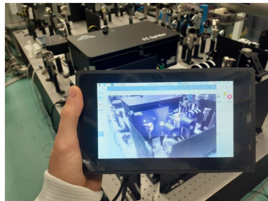
Figure 1.7.6: Example of using the Raspberry Pi IR-viewer in E4. Following the laser at wavelength of 1064 nm.
