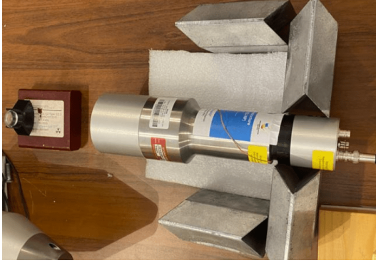
Figure 4.3.8: Experimental setup for the characterization of CeBr 3 detectors.
