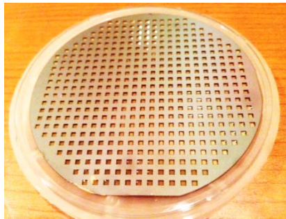
Fig. 45 – Si wafer with approximately 1000 ultra-thin SiN windows to be manufactured in the ELI-NP Target Fabrication Laboratory.
