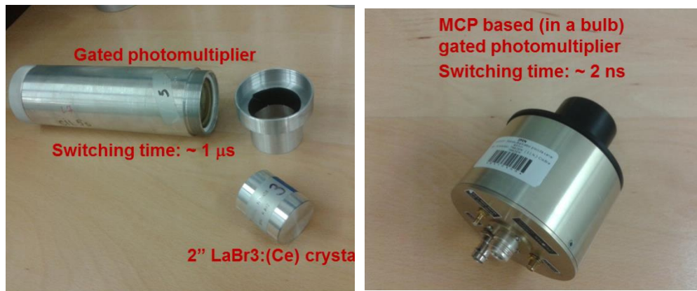
Figure 36 – Left: Dynode based gated-photomultiplier and LaBr 3 crystal scintillator. Right: same crystal coupled to an MCP based photomultiplier
