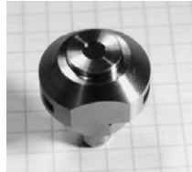
Fig. 36 – ^{22}\text{Na} capsule (iThemba) to be used as e^+ source.
