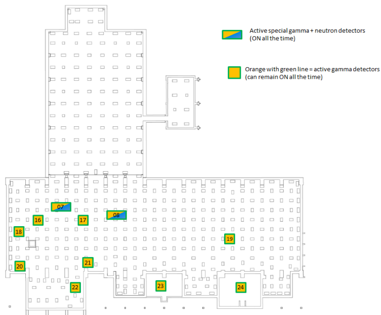
Fig. 17 - Position of active area monitors in the basement.
